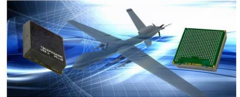
These drives are complete with an SSD controller based on a 32-bit RISC processor and 4 NAND flash memory devices. High performance is provided by concurrent access of multiple Flash channels and support for performance features such as Native Command Queuing.
